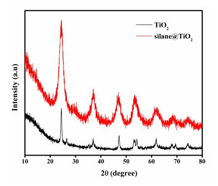
Figure 2. XRD pattern of TiO<sub>2</sub> and silane@TiO<sub>2</sub> nanoparticles.
