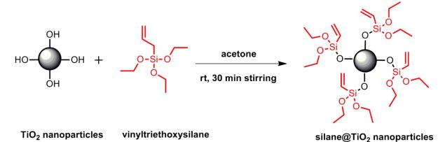
Scheme 1. Schematic route for the synthesis of the silane@TiO<sub>2</sub> nanoparticles.
