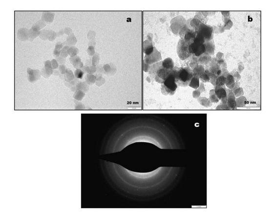
Figure 5. (a, b) TEM images  $TiO_2$  and  $silane@TiO_2$  nanoparticles. (c) Selected area electron diffraction pattern of silane@TiO\_2 nanoparticles.
