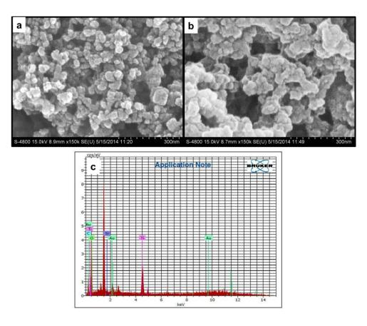
**Figure 3.** (a, b) FE-SEM images of  $TiO_2$  and silane@TiO<sub>2</sub> nanoparticles, (c) EDX spectrum of silane@TiO<sub>2</sub> nanoparticles.
