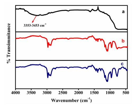
Figure 1. FT-IR spectrum of (a) TiO<sub>2</sub>, (b) silane@TiO<sub>2</sub>, (c) vinyltriethoxysilane.
