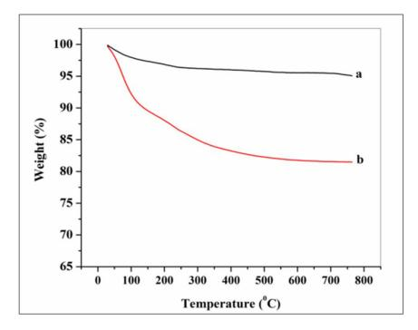
**Figure 4.** TGA thermograms of (a)  $TiO_2$  and (b) silane@TiO<sub>2</sub> nanoparticles under nitrogen atmosphere at a heating rate of 10 °C/min.
